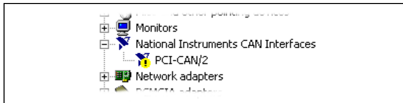
Figure C-1. CAN Interface That Is Not Working Properly
